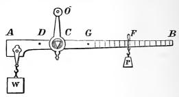
AB is an iron bar turning about the edge C of a triangular piece of metal, which works in an aperture of the handle by which the balance is suspended from a point O.
